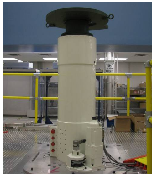
Figure 1 - The retracted mast is designed to fit within the host platform with the mounted sensor resting near the vehicle roof line
