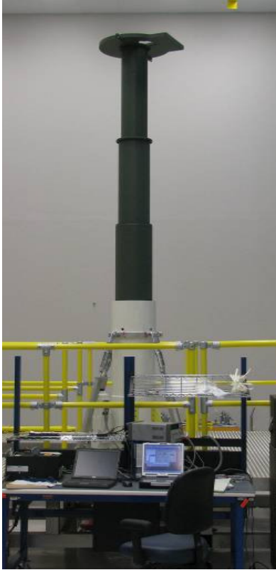
Figure 2 - The extended mast provides long range line-of-sight to a mounted sensor while the vehicle itself can remain hidden in defilade or behind an obscuring wall or low tree line
